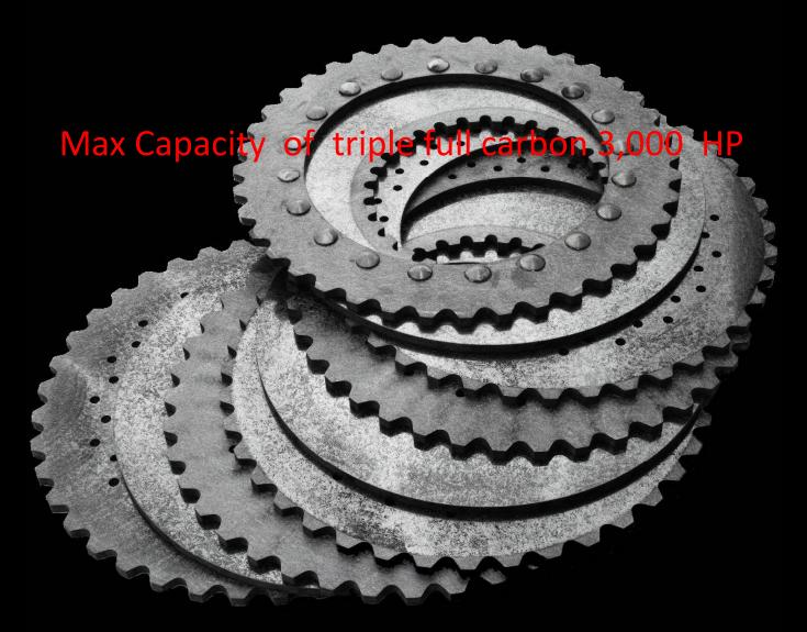
Based on the test result, the first maintenance would be just adding one shim after about 500 drag launces. (Please not e that this is a simple calculation based on the test we had. The result would vary depending on several conditions on the car and road condition.)
